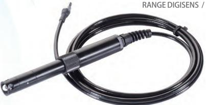
The PHEH sensor has been designed to perform under hard conditions from pure mountains water with conductivity as low as 20  $\mu$ S/cm, lakes and rivers (100 - 2000  $\mu$  S/cm), seawater with conductivities of 50 mS/cm and to wastewater with conductivity higher than 200 mS/cm.
